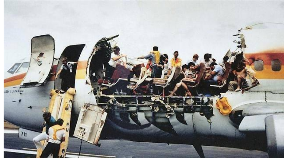
1988: Aloha Airlines Flight 243 Fatigue-cracking in lap-joint
